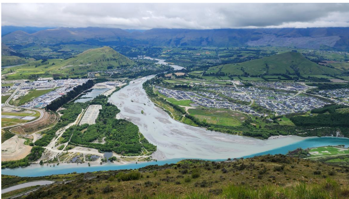
Figure 10: Lower Shotover River and Shotover Wastewater Treatment (WWTP) area and disposal field on 3 rd December 2025, the day before the survey. This image illustrates the flood prone nature of the delta area in a flow of just 64.1\text{m}^3/\text{s} recorded EM215 NIWA Shotover at Bowen Peak at 11:00am, 10 minutes prior to this photo. Following high flows (refer Table 2 in Appendix 2), the river tends to flow high over the new gravel beaches deposited by the bedload until the flow can incise braids into them. Photo ref: D Palmer 20251203_111059
